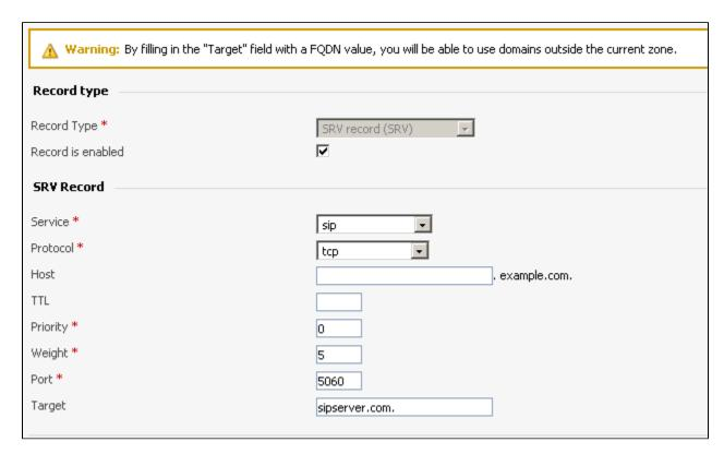
This points to a server named sipserver.com listening on TCP port 5060 for SIP protocol services. The priority given here is 0 and the weight is 5.
