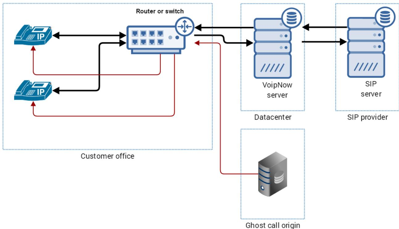
**The black arrows** indicate the regular call traffic: your customer's phones are connected to the router/switch installed in the office, then to the VoipNow server which in turn connects to the SIP provider's server.
