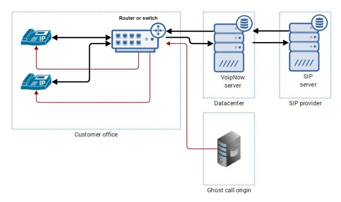
The black arrows indicate the regular call traffic: your customer's phones are connected to the router/switch installed in the office, then to the VoipNow server which in turn connects to the SIP provider's server.
